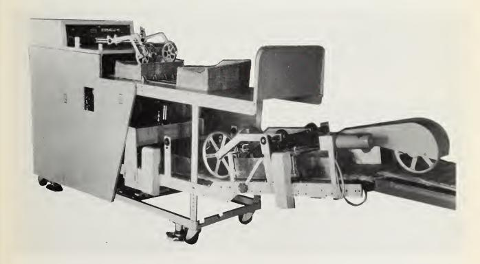
PRESS ACCESSORY MONITORS SHEET GUIDING — The "Side Guide Detector System" employs two photo cell sensors to monitor the two side guiding mechanisms on the feed boards of most printing presses. Intended for use with all kinds of sheet stock, this compact unit can be set to sound an alarm or stop the press if five consecutive sheets are misguided. Price range is \$890-990. WRITE: Gordon W. Wilson, Electro Sprayer Systems, Inc., Dept. CN, 5423 Milton Parkway, Rosemont, Illinois 60018 U.S.A.
